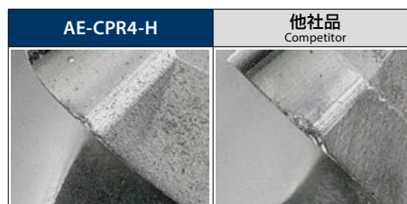
1,512m 加工後の刃先の損傷状態 Wear comparison of the cutting edge after milling 1,512 m
