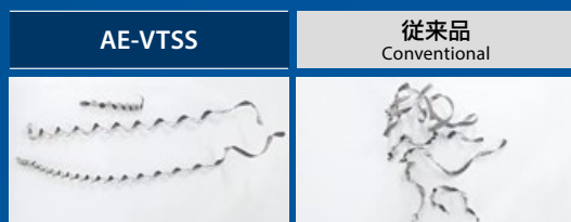
突込み加工時の切りくず形状 Chip shape from plunging
