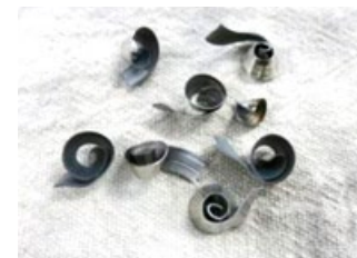
P3Dの切りくず Cutting Chips of P3D
